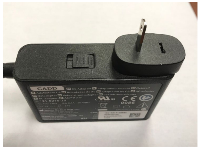
Figure 2: AC Adapter with Missing AC Prong
