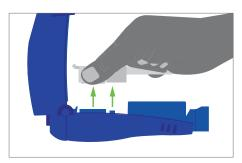
Detach the rocker assembly by placing your forefinger and thumb on either side of the grooved surface and gently lift the rocker up.
