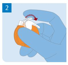
Release trigger lock mechanism by pushing down the screw button.
